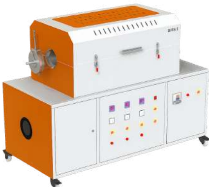
Vacuum Heat Treatment Furnace (Annealing, Sintering, Brazing. etc.) (600 °C - 1600 °C)
