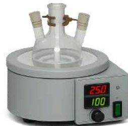
Liquid Precursor Generator (RT to 200 °C)
