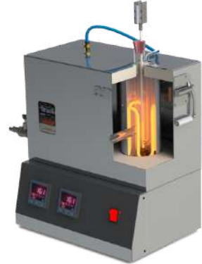
CPT Furnace (Up to 350 °C)
