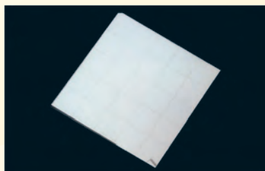
Alumina 96% with Laser Striations at 19mmx19mm
